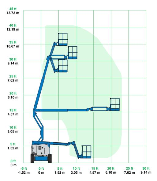
\*The metric equivalent of working height adds 2 m to platform height. Imperial adds 6 ft to platform height. \*\*In lift mode (platform raised) the machine is designed to operate on firm, level surfaces only. \*\*\*Gradeability applies to driving on slopes. See operator's manual for details regarding slope rating. \*\*\*\*Floor loading information is approximate. It should be used only with adequate safety factors. \*\*\*\*Weight will vary depending on options.
